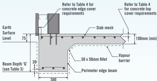
FIGURE 6 - TYPICAL SECTION THROUGH EDGE PERIMETER BEAM
