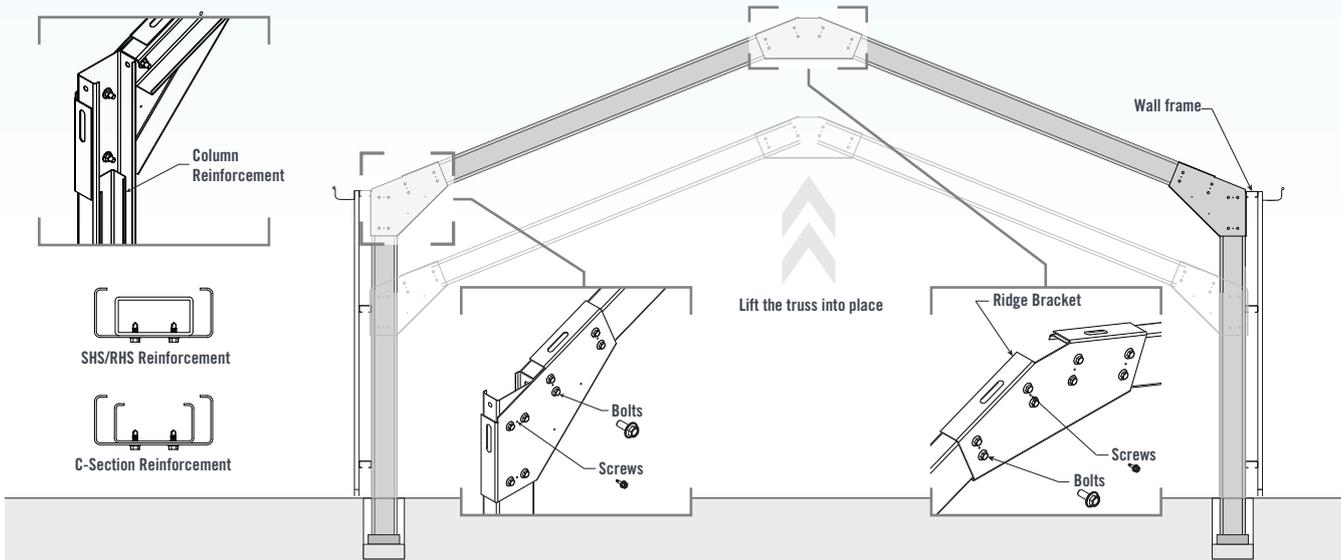
**PORTAL FRAME ASSEMBLY - ALTERNATIVE ROOF PITCHES**
