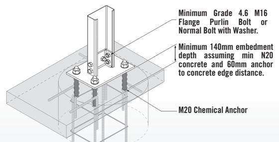
INTERNAL COLUMN WITH SLAB
